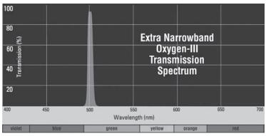
This graph shows the typical light transmission through the Orion Oxygen-III filter. Note that the filter only passes visible light with wavelengths between 485nm and 515nm with a full width half maximum value of approximately 7nm. All other wavelengths are essentially blocked. Transmission is greatest at 500.7nm, which is the Oxygen-III emission wavelength.
