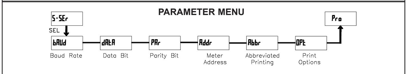
The Serial Setup Parameters are only active when the optional RS232 or RS485 serial communications module is installed in the meter. Refer to the DP6-COM bulletin for complete details on DP63000 serial communications.
