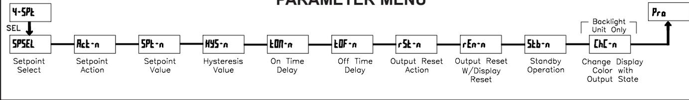
The Setpoint Output Parameters are only active when an optional output module is installed in the meter.
