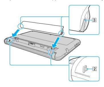
4 Push the battery pack down into the compartment until it clicks into place.
