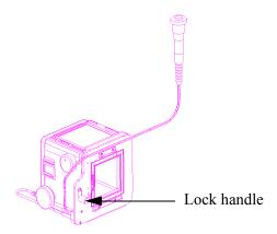
3. Turn the lever on the Cable Release plug to O. (Refer to the picture on page 3.) Insert the plug into the auxiliary release jack on the front of the RZ67, then turn the lever to L to lock the plug. (When removing the cable, turn the lever from L to O and pull the plug out.)
