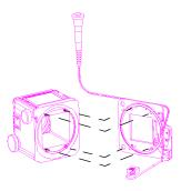
2. Slide the Lock handle downward to secure the plate to the camera body.
