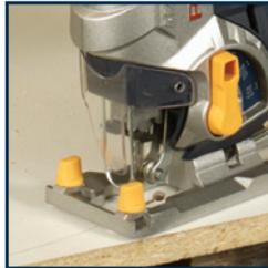
**WARNING.** Do not move the saw forward along its cut until the blade has completely entered the material and the shoe comes to rest on its surface.
