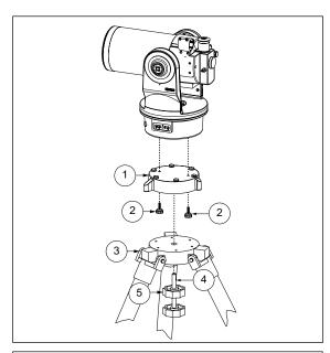
Figure 1: Alt-Az Assembly. Item 1: Adapter; Item 2: Adapter Knobs; Item 3: Tripod; Item 4: Threaded Rod; Item 5: Tension Lock Nut.
