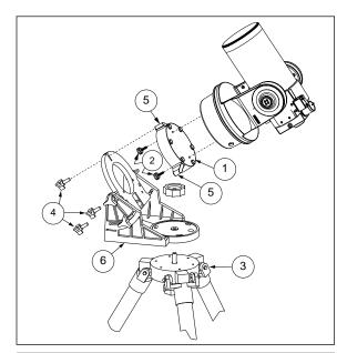
Figure 2: Polar Assembly. Item 1: Adapter; Item 2: Adapter Knobs; Item 3: Tripod; Item 4: Tab Knobs; Item 5: Tabs; Item 6: Equatorial Wedge.
