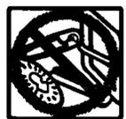
Do not put sharp or metal objects in your washer. They can damage the finish. Check all pockets for pins, clips, money, bolts, nuts, etc.
