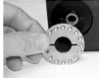
With the disc removed, a different disc can be inserted to change the angular spacing. The 14 position detent disc (included with your bracket) is for use with the optional Olympus Wide Conversion Lens WCON-08.
