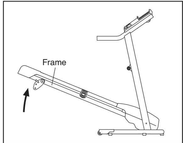
2. Move your right hand to the position shown and hold the treadmill firmly. Using your left hand, pull the latch knob to the left and hold it. Raise the frame until the latch plate is past the latch pin. Then, slowly release the latch knob; make sure that the latch plate is resting against the latch pin.
