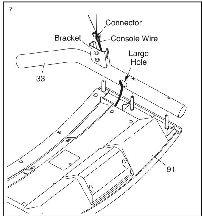
8. Set the Right Handrail (33) on the Console (91). **Make sure that the console wire is not pinched.** Start a 16mm Screw (85) with an M5 Star Washer (7) into the Right Handrail, and then start two 19mm Screws (10) into the Right Handrail. **Tighten the 16mm Screw and then tighten the two 19mm Screws; do not over-tighten the Screws.**
