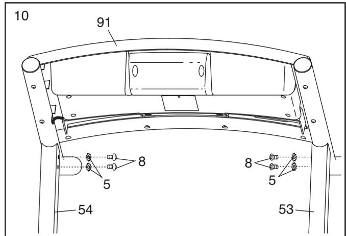
11. Start an M8 x 15mm Bolt (8) with an M8 Star Washer (5) into each Upright (53, 54). **See steps 10 and 11. Firmly tighten all six M8 x 15mm Bolts.**
