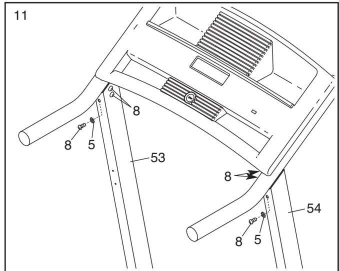
12. Lower the Uprights (53, 54). **See the lower drawing.** Position the Uprights so that the treadmill Frame (51) is centered between the Uprights.
