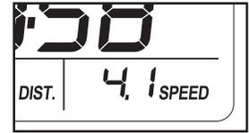
**The upper display**—The upper display can show the elapsed time, the distance that you have walked or run, the speed of the walking belt, or the approximate number of calories you have burned. Press the Display button repeatedly until the upper display shows the information that you are most interested in viewing. Note: While information is shown in the upper display, the same information will not be shown in the lower displays.
