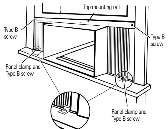
**NOTE:** Seal any openings around the case or accordion panels with sealer or foam gaskets.
