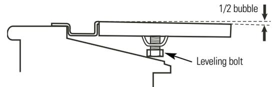
**NOTE:** Use a steel washer between the leveling bolts and the sill if the sill is weak.
