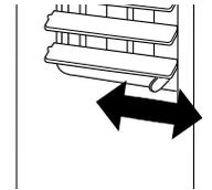
*To open the vent, push the lever to the right.
