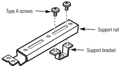
**NOTE:** The support bracket may be attached into either slot in the support rail, depending on the depth of your window sill.
