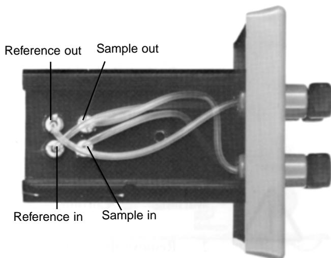
**Fig. 13.** Flow cell interior showing tubing connections.
