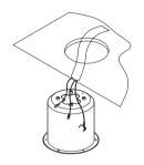
Connect the cables to the video cable terminal and controller cable terminal on the circuit board of the mounting bracket.
