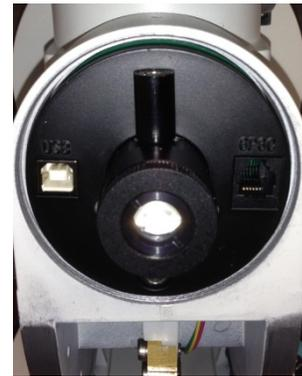
Figure 23. Polar Scope LED
