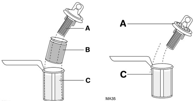
3. Turn the handle about 1/4 a turn anticlockwise and remove.
