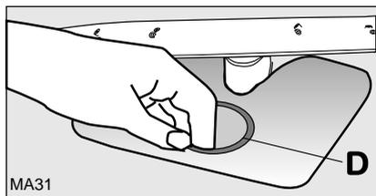
7. Put the flat filter (D) back in the base of the washing compartment.
