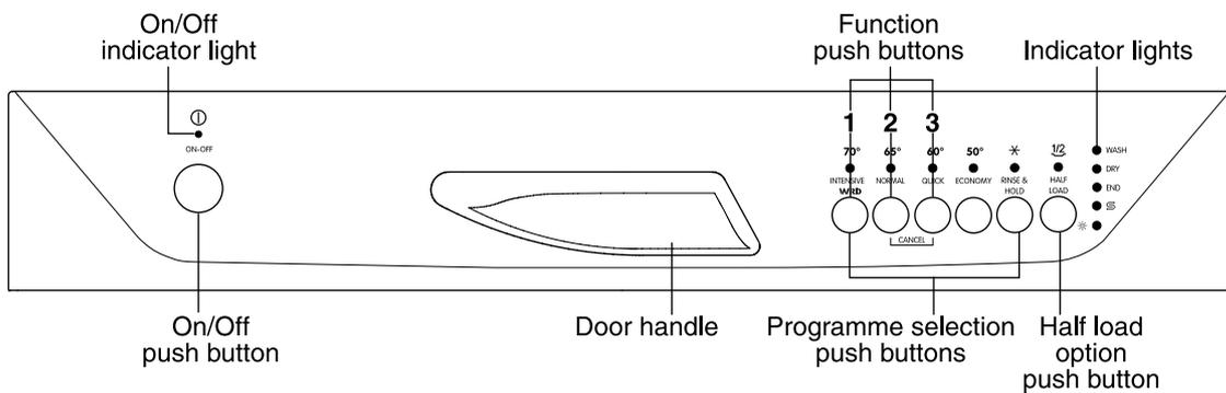
**Function push buttons:** in addition to the dishwashing programme selected, the following functions can also be set with the help of these buttons: water softener setting, deactivation/activation of the inflow of rinse aid and the cancelling of a programme in progress.
