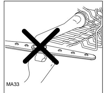
Check that the WRD is not clogged with detergent residue. If necessary rinse it under running water after having removed it from the basket by twisting it anticlockwise and pulling it upwards.
