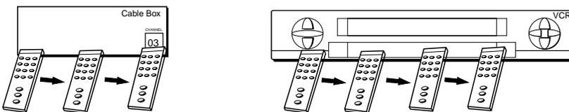
4. When the component turns on, you've located the remote control sensor.
