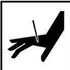
**Do not load nails with the trigger or safety depressed.** Unintentional firing may occur. Do not load nails when the air hose is connected to the tool. Always assume the tool contains nails.
