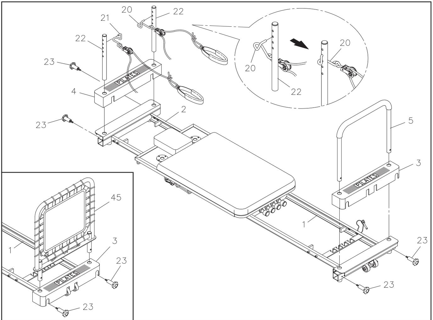
**STEP 5:** Remove the paper covering from the foam tape inside the **FRONT COVER(3)** and **REAR COVER(4)**. Place the **FRONT COVER(3)** over the **FRONT FRAME(1)**. Place the **REAR COVER(4)** over the **REAR FRAME(2)**. Press the covers securely in place.
