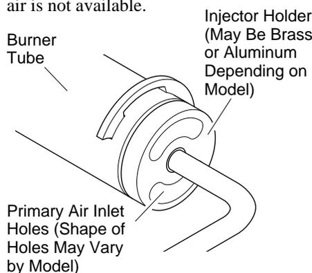
**Figure 27 - Injector Holder On Outlet Burner Tube**
