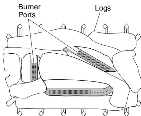
**Figure 18 - Installing Log set (Top View)**
