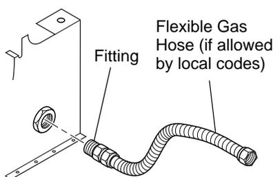
**Figure 11 - Attaching Flexible Gas Hose to Heater**
