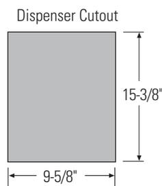
\*Cut the dispenser opening after the backer, spacer and overlay panels have been assembled.
