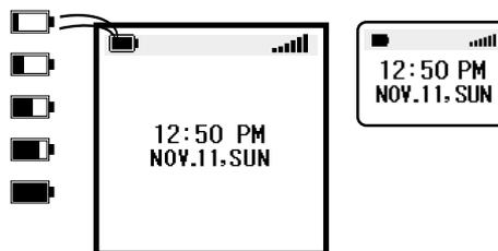
The phone will automatically switch **OFF** shortly after the empty battery symbol starts flashing and **'LOW BATTERY'** appears on display. You can clear the message temporarily by pressing any key.
