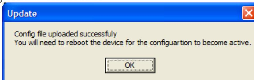
By design, the IP Address configuration currently on the device is kept intact and not overwritten by the new configuration file.
