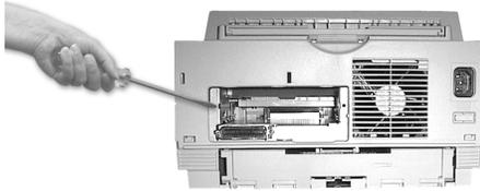
Use a screwdriver to remove serial interface board from back panel of printer.
