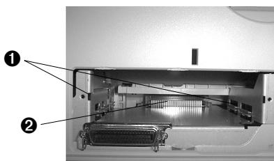
Locate guide rails ❶ and edge connector ❷.
