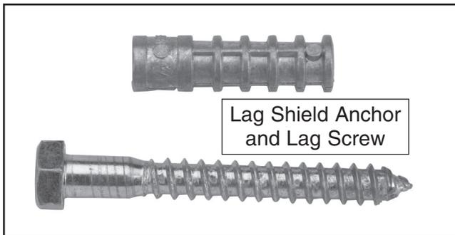
Installation of lag shields requires holes to be drilled into the concrete to accommodate them. Drilling into concrete properly requires a hammer drill with an appropriate sized concrete drill bit.
