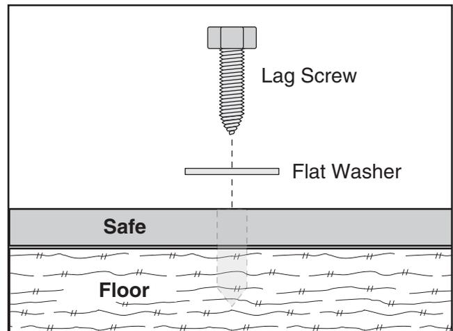
Installation works best if holes are pre-drilled to accommodate the lag screws. A standard hand-held power drill with the appropriate-sized wood drill bit is required to complete the job.
