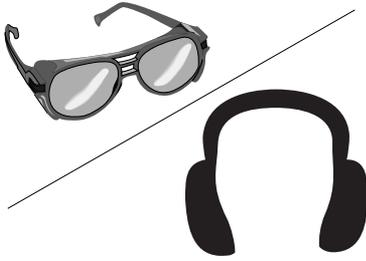
Operating this nailer can propel objects into the air, causing immediate eye damage. To protect yourself, always wear American National Standards Institute (ANSI) approved safety glasses or goggles when operating this equipment. In addition, this nailer discharges at approximately 85-90 decibels. To protect your hearing, always wear ANSI approved ear protection when operating.
