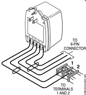
1. Splice one end of a 3-conductor cable to the wire ends of the SA4120XM-1 Cable.
