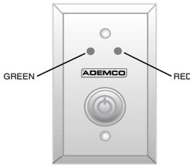
1. Connect the 4146 keyswitch's normally open momentary switch to a zone's (2-8) terminals. Remove the 2000 ohm EOL resistor if connected across the selected zone.
