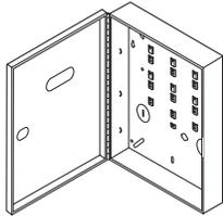
1. Mount the control cabinet to a sturdy wall in a clean, dry area, which is not readily accessible to the general public, using fasteners or anchors (not supplied) with the four cabinet mounting holes.
