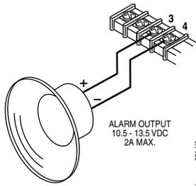
Make sounder connections to alarm output terminals 3 (+) and 4 (-).
