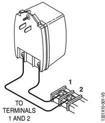
Connect the 1321 Transformer (1321CN in Canada) to terminals 1 and 2 on the control board. See Wire Run Chart for wire size to use.
