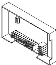
1. Connect each module to the control’s keypad terminals and set the device addresses.
