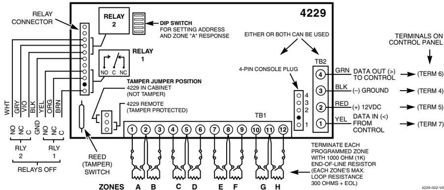
Figure 10. Wiring Connections, 4219 & 4229 (4229 shown)
