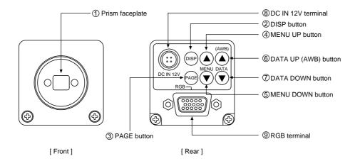
1 Prism faceplate The protection cap is attached on the lens mount portion. After removing the cap, mount the lens. Be careful not to scratch or touch the optical area.
