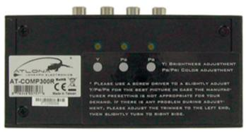
\* Please use a screw driver to a slightly adjust Y/Pb/Pr for the best picture in case the manufacturer presetting is not appropriate for your demand. If there is any problem during adjustment, please adjust the trimmer to the left end, then slightly turn to right side.
