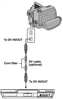
Video unit equipped with DV connector
