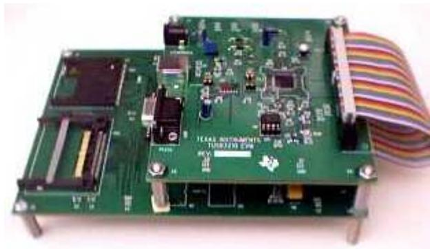
Figure 1–4. TUSB3210 Printed-Circuit Board (REV 1.1)—Top Side
