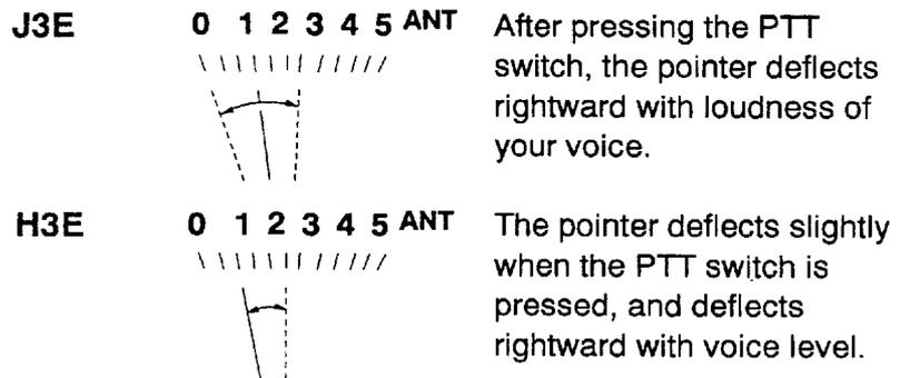
**NOTE:** *The LCD shows “antenna current”. The pointer deflecting range differs by frequency or antenna length.*
