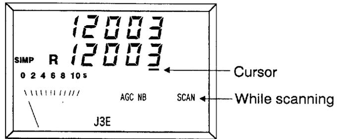
3. To stop scanning, press the **SCAN** key or the **PTT** switch. “SCAN” disappears from the LCD.
