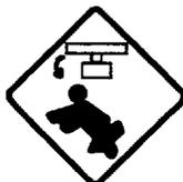
**Wear a safety belt and a hard hat when working high up on the mast or close to the radar antenna. Do not look into the radar antena at a close distance.** Stop the radar while working with the radiotelephone antenna.
