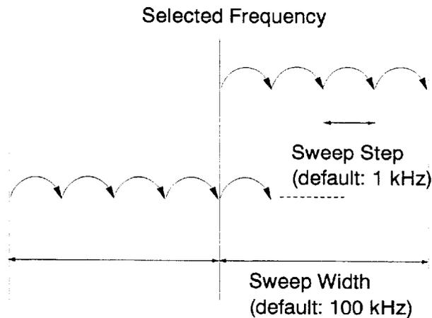
**NOTE:** Sweep width is the frequency width to sweep on both sides of the selected frequency.
