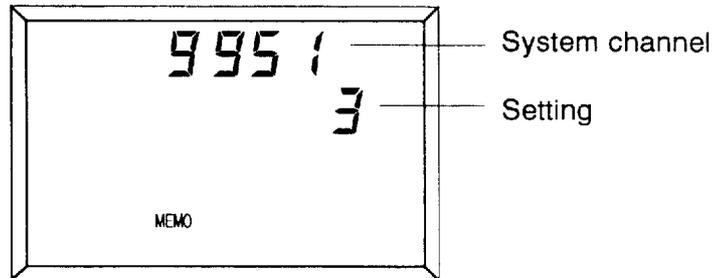
2. Turn the **FREQ/CH** encoder to select a desired channel number.
