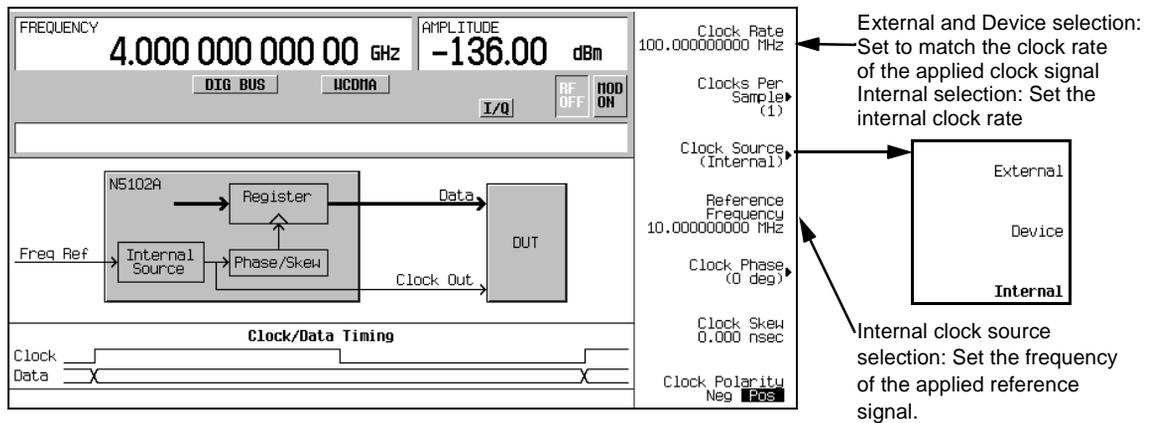
When you select a clock source, you must let the N5102A module know the frequency of the clock signal using the **Clock Rate** softkey. In the internal clock source mode, use this softkey to set the internal clock rate. For device and external clock sources, this softkey must reflect the frequency of the applied clock signal.
