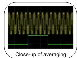
The ALC samples the waveform when the marker signal goes high, and uses the average of the sampled waveform to set the ALC circuitry.
