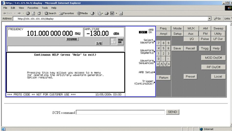
This web page remotely accesses all signal generator functions and operations. Use the mouse pointer to click on the signal generator's hardkeys and softkeys. The results of each mouse click selection will be displayed on the web page. For example, click on the Frequency hardkey then use the front-panel key pad to enter a frequency. You can also use the up and down arrow keys to increase or decrease the frequency.
