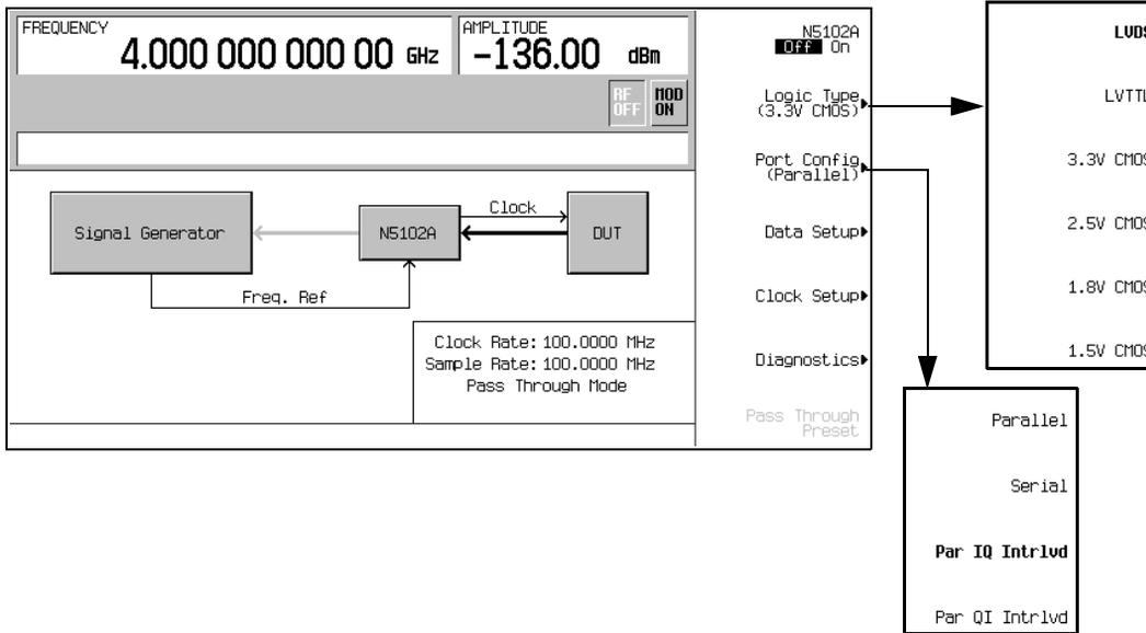
1. Refer to [Figure 11-16](#). Press the **Logic Type** softkey.
