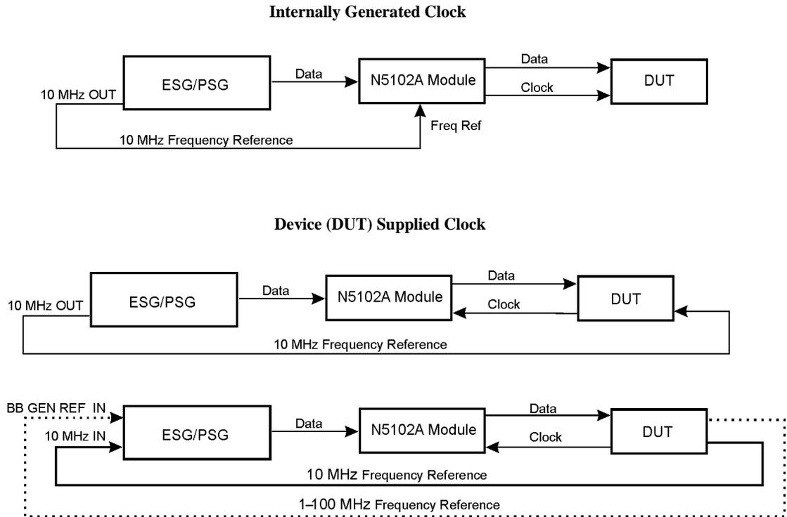
**NOTE:** Use only one of the two signal generator frequency reference inputs.
