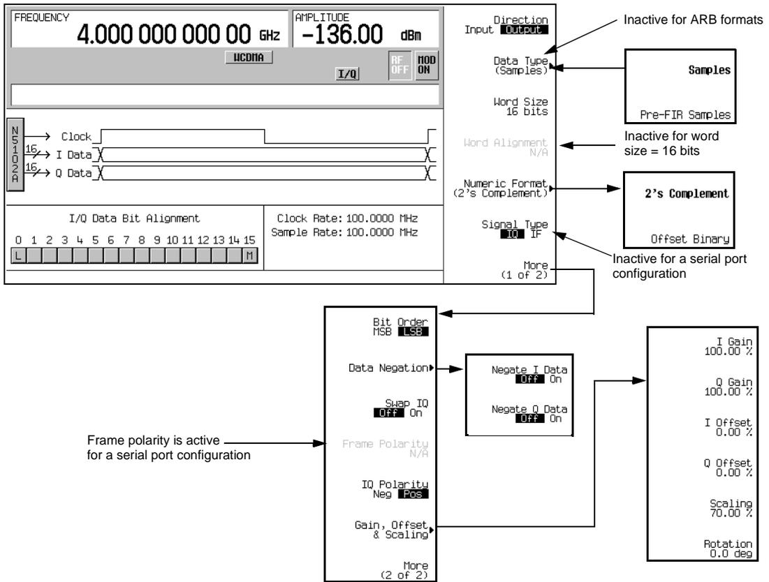
2. If a real-time modulation format is being used, press the **Data Type** softkey. (This softkey is inactive when an ARB modulation format is turned on.)
