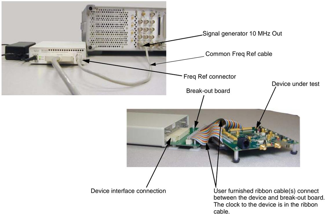
1. Refer to the five setup diagrams in [Figure 11-3 on page 209](#) and connect the frequency reference cable according to the clock source.
