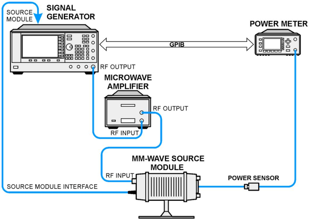
Figure 4-6 User Flatness with mm-Wave Source Module and Option 1EA Signal Generator
