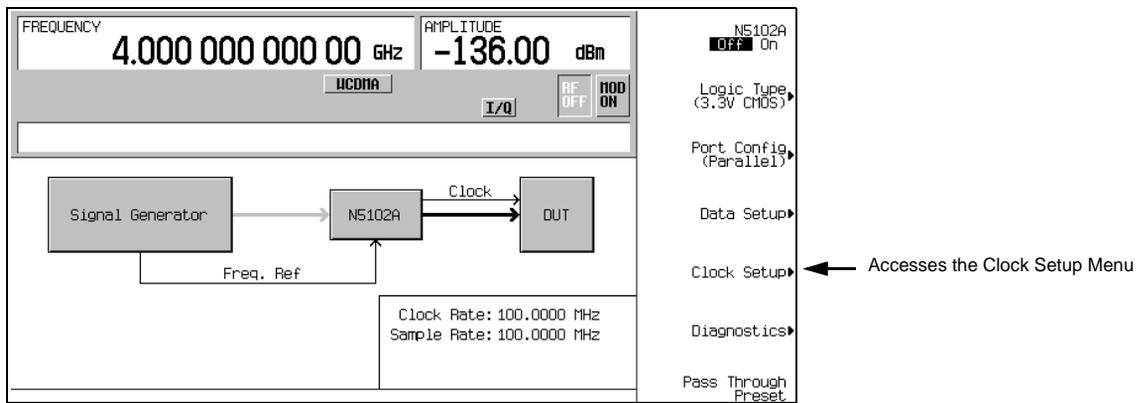
From this softkey menu, set all of the clock parameters that synchronize the clocks between the N5102A module and the PSG. You can also change the clock signal phase so the clock occurs during the valid portion of the data. Figure 11-14 shows the clock setup menu.
