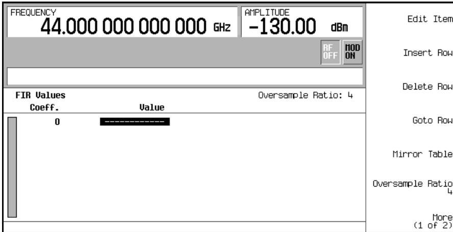
5. Press **Edit Item**. The value field for coefficient 0 should be highlighted.
