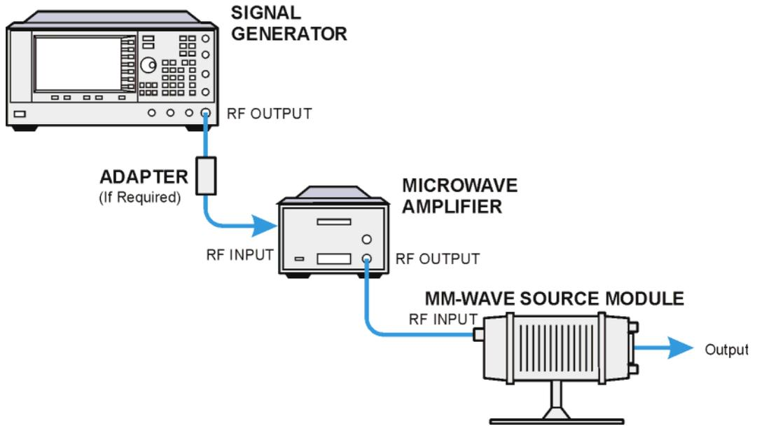
Figure 11-24 Setup for E8267D PSG and E8257D PSG with Option 1EA
