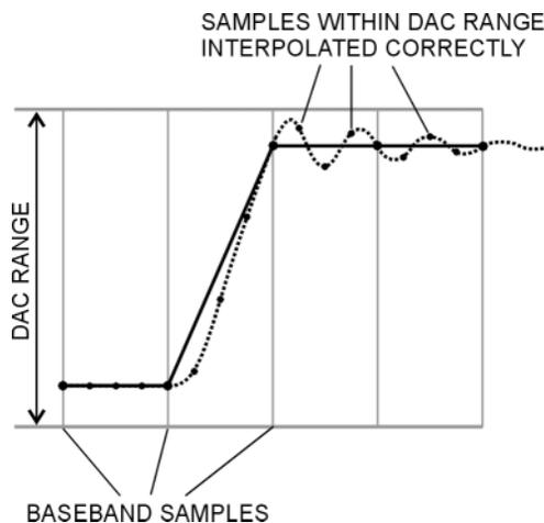
Although scaling maintains the basic shape of the waveform, too much scaling can compromise its integrity because the bit resolution can be so low that the waveform becomes corrupted with quantization noise. Maximum accuracy and optimum dynamic range are achieved by scaling the waveform just enough to remove the DAC over-range error. Optimum scaling varies with waveform content.
