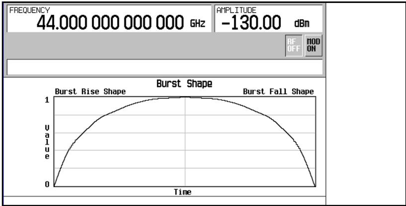
**NOTE** To return the burst shape to the default conditions, press **Return > Return > Confirm Exit From Table Without Saving > Restore Default Burst Shape**.
