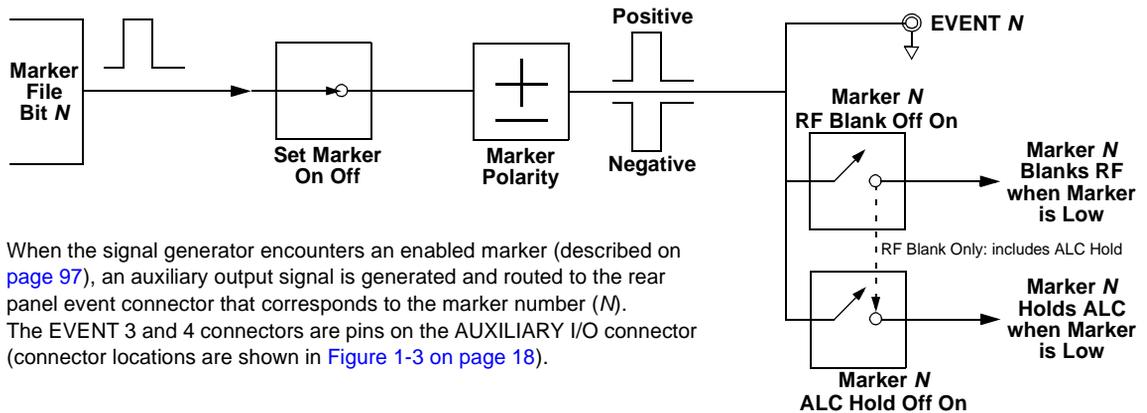
When the signal generator encounters an enabled marker (described on [page 97](#)), an auxiliary output signal is generated and routed to the rear panel event connector that corresponds to the marker number ( $N$ ). The EVENT 3 and 4 connectors are pins on the AUXILIARY I/O connector (connector locations are shown in [Figure 1-3 on page 18](#)).
