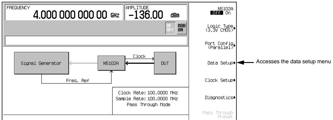
This softkey menu accesses the various parameters that govern the data received by the PSG. The status area of the display shows the number of data lines used for both I and Q along with the clock position relative to the data. [Figure 11-20](#) shows the data setup menu structure.
