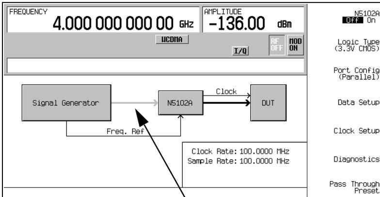
Line is grayed out until the N5102A module interface is turned on
