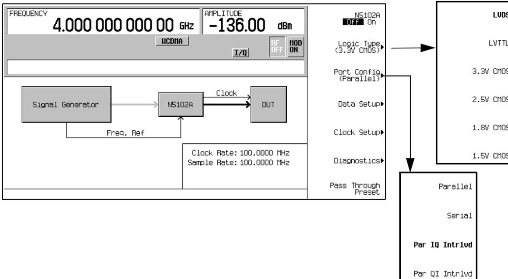
1. Refer to [Figure 11-10](#). Press the **Logic Type** softkey.
