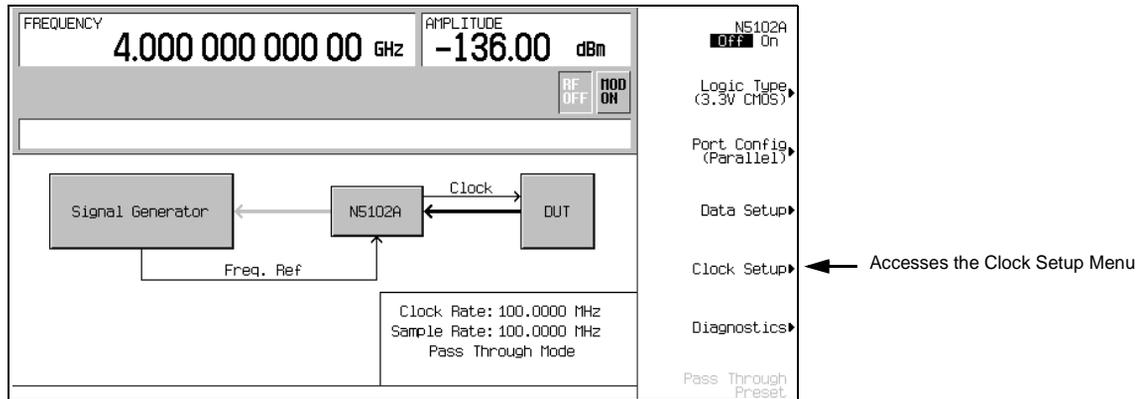
From this softkey menu, set all of the clock parameters that synchronize the data between the N5102A module and the device. From this menu, the clock signal phase can be changed so the clock occurs during the valid portion of the data. [Figure 11-18](#) shows the clock setup menu.
