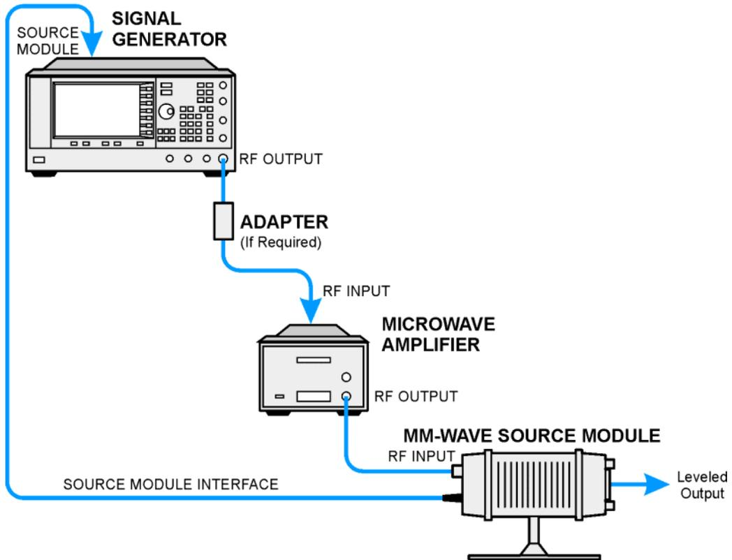
Figure 11-22 Setup for E8267D PSG and E8257D PSG with Option 1EA
