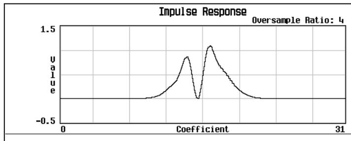
The graphic display can provide a useful troubleshooting tool (in this case, it indicates that a coefficient value is set incorrectly, resulting in an improper Gaussian response).
