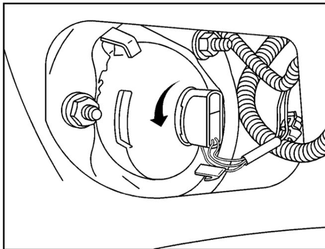
3. Turn the bulb socket counterclockwise and pull it out of the lamp assembly.
