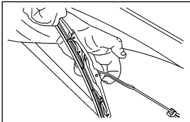
2. Push the release lever and slide the wiper assembly toward the driver side of the vehicle.
