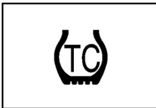
This indicator comes on whenever the vehicle Traction Control system is actively working.
