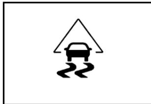
For vehicles with the Electronic Stability Control (ESC) system or the Traction Control System (TCS), the indicator/warning light comes on briefly when the engine is started.
