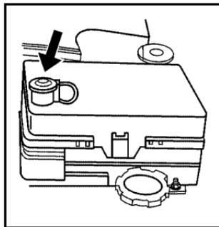
Locate the remote positive (+) terminal which is located under a red tethered cap on the engine compartment fuse block. Lift the cap to access the terminal.
