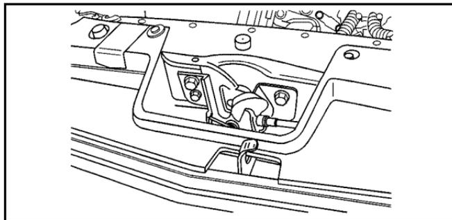
2. Then go to the front of the vehicle and push the secondary hood release lever to the left. It is located under the front center of the hood toward the driver's side of the vehicle.
