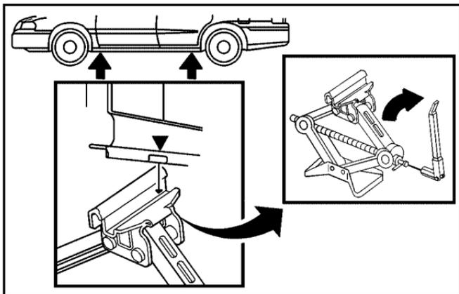
5. Position the jack lift head at the jack location nearest the flat tire. The front location is about 8 inches (20 cm) behind the front wheel opening. The rear location is about 4 inches (10 cm) in front of the rear wheel opening.
