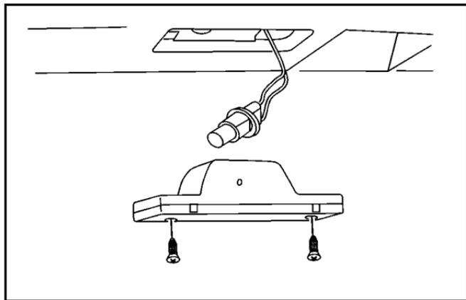
1. Remove the two screws holding each of the license plate lamps.
