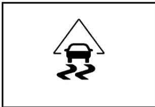
When this light is on and either the SERVICE TRACTION or TRACTION OFF message is displayed, the system will not limit wheel spin.
