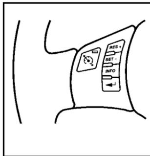
The cruise control buttons are located on the outboard side of the steering wheel.
