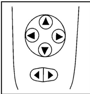
Controls for the outside power mirrors are located on the driver door armrest.
