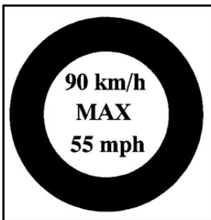
15. If the flat tire was able to inflate to the recommended inflation pressure, remove the maximum speed label from the sealant canister (B) and place it in a highly visible location.
