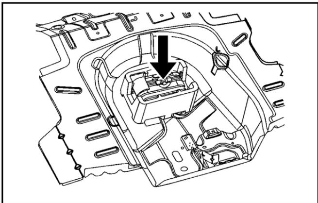
3. Remove the retainer that holds the tire sealant and compressor kit.
