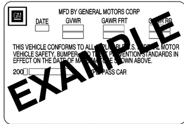
A vehicle specific Certification label, found on the rear edge of the driver door, tells you the gross weight capacity of your vehicle, called the Gross Vehicle Weight Rating (GVWR).
