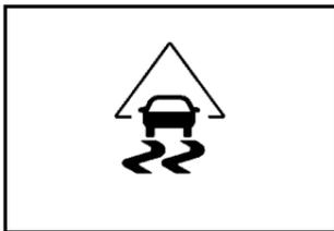
For vehicles with the Enhanced Traction System (ETS), this light serves as an indicator and warning light.
