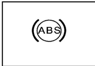
For vehicles with the Antilock Brake System (ABS), this light comes on briefly when the engine is started.
