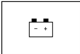
This light comes on briefly when the ignition is turned on, and the engine is not running, as a check to show it is working. Then it should go out when the engine is started.
