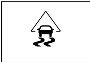
This light flashes on the instrument panel cluster when the ESC system is on and activated.
