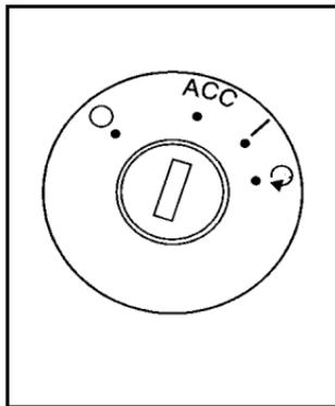
The ignition switch has four different positions.
