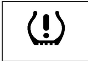
When a low tire pressure condition is detected, the TPMS turns on the low tire pressure warning light located on the instrument panel cluster.
