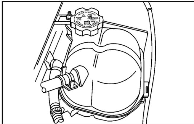
The coolant surge tank is located in the engine compartment on the driver's side of the vehicle. See *Engine Compartment Overview* on page 6-14 for more information on location.
