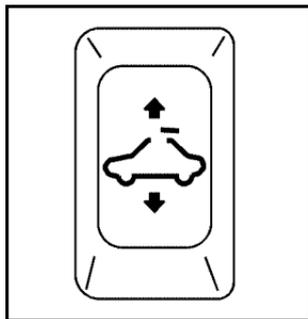
On vehicles with a sunroof, the switch that operates it is located on the headliner between the map lamps.
