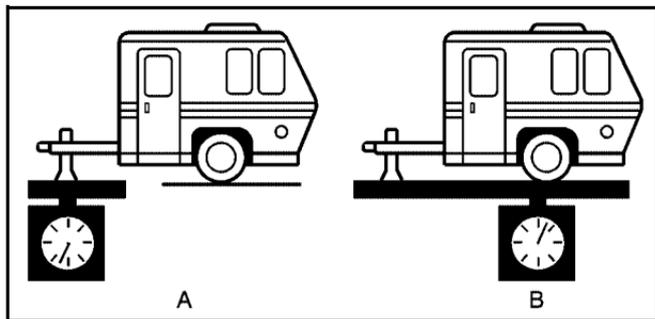
If using a weight-carrying hitch, the trailer tongue (A) should weigh 10 to 15 percent of the total loaded trailer weight (B).
