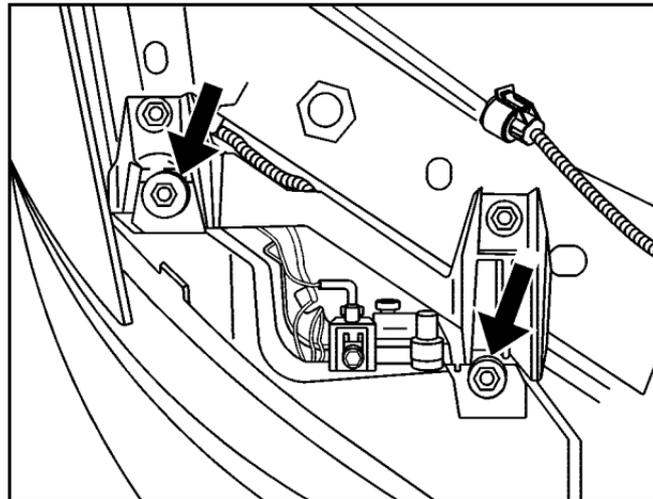
2. Remove the two bolts from the headlamp assembly.
