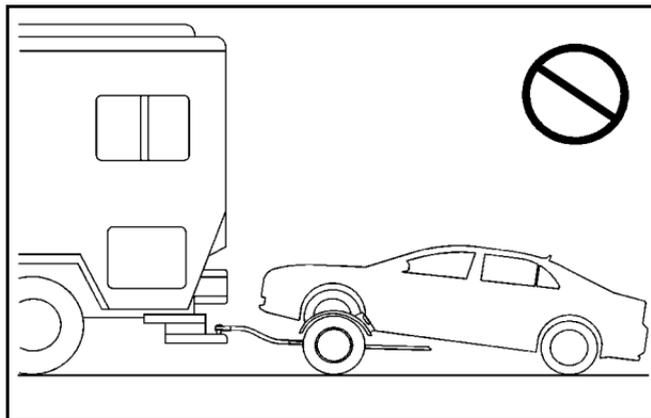
The vehicle cannot be dolly towed, but can be dinghy towed. See “Dinghy Towing” earlier in this section.
