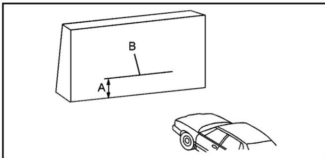
3. At the wall, measure from the ground upward (A) to the recorded distance from Step 2 and mark it.
