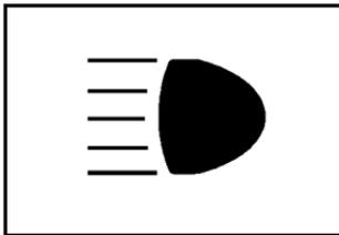
This indicator light appears on the instrument panel cluster when the high beams are on.
