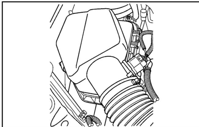
To inspect or replace the filter, remove the screws that hold the cover on and lift off the cover. Be sure to reinstall the cover tightly.
