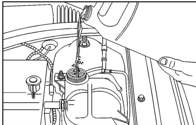
3. Fill the coolant surge tank with the proper mixture, to the COLD FILL line on the tank. Wait about five minutes, then check to see if the level is below the COLD FILL line. If the level is below the line, add additional coolant to bring the level up to the line. Repeat this procedure until the level remains constant at the COLD FILL line for at least five minutes.
