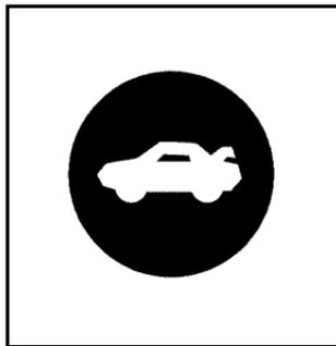
To open the trunk from inside the vehicle, press the remote trunk release button. It is located inside the driver storage compartment on the lower left side of the instrument panel.
