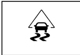
This indicator comes on whenever the vehicle StabiliTrak<sup>®</sup> is actively working.
