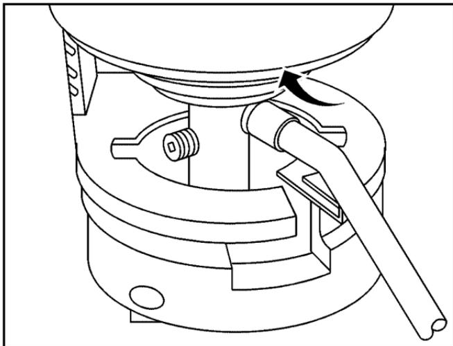
4. Turn the sealant canister (B) so the inflator filling hose is aligned with the slot in the compressor.
