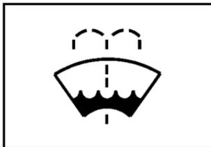
Open the cap with the washer symbol on it. Add washer fluid until the tank is full. See *Engine Compartment Overview* on page 6-14 for reservoir location.
