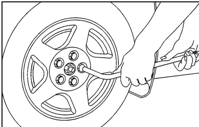
2. If your vehicle has plastic wheel covers, use the wheel wrench to loosen the plastic wheel nut caps. Once the plastic wheel nut caps have been loosened with the wheel wrench, you can finish loosening them with your fingers. The plastic nut caps do not come off.
