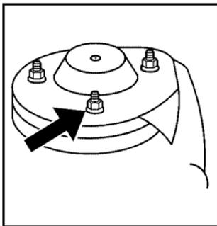
Locate the remote negative (-) ground terminal, marked GND (-), which is located behind the engine coolant surge tank.
