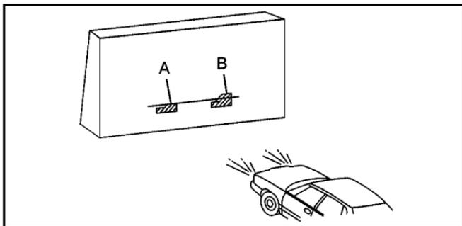
8. Make sure that the light from the headlamp is positioned at the bottom edge of the horizontal tape line. The lamp on the left (A) shows the correct headlamp aim. The lamp on the right (B) shows the incorrect headlamp aim.
