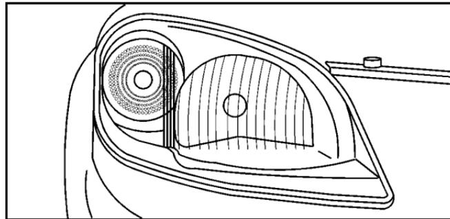
2. Record the distance from the ground to the aim dot on the low-beam headlamp.
