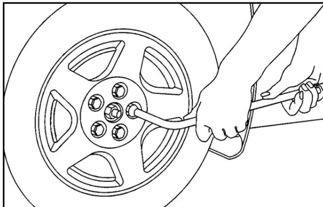
3. If your vehicle has plastic wheel covers, use the wheel wrench to loosen the plastic wheel nut caps. Once the plastic wheel nut caps have been loosened with the wheel wrench, you can finish loosening them with your fingers. The plastic nut caps do not come off.
