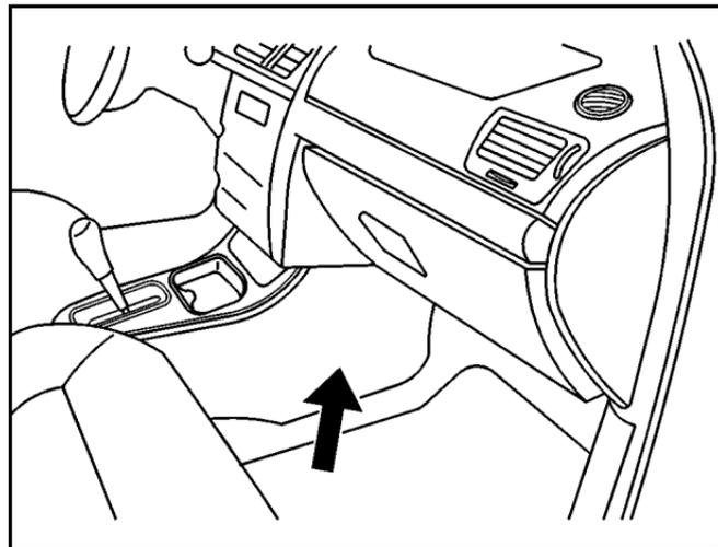
The floor console fuse block is located on the passenger side of the floor console behind the forward panel. The panel has three clips. Pull the panel to disconnect the three clips, and access the fuses. Use the fuse puller to remove fuses.
