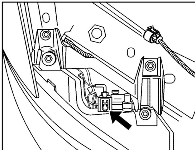
6. Locate the vertical headlamp aiming screws, which are under the hood near each headlamp assembly. The adjustment screw can be turned with a 6 mm socket wrench.
