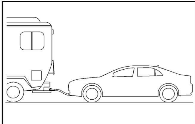
The vehicle may be dinghy towed from the front with all four wheels on the ground following these steps:
