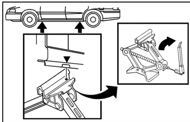
5. Position the jack lift head at the rear jack location nearest the rear tire. The rear location is about 4 inches (10 cm) in front of the rear wheel opening.
