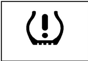
The Tire Pressure Monitor alerts you when a significant reduction in pressure occurs in one or more of the vehicle's tires by illuminating the low tire pressure warning light on the instrument cluster.
