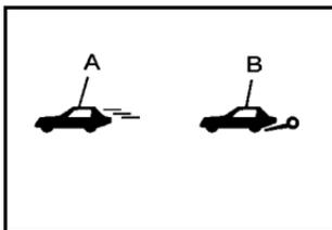
This indicator comes on when Competitive Driving Mode (A) has been set using the traction control switch. This telltale comes on whenever conditions are right for the Launch Mode (B) to activate.
