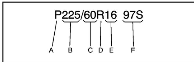
**(A) Passenger (P-Metric) Tire:** The United States version of a metric tire sizing system. The letter P as the first character in the tire size means a passenger vehicle tire engineered to standards set by the U.S. Tire and Rim Association. A tire size without the letter P as the first character is certified to European standards.
