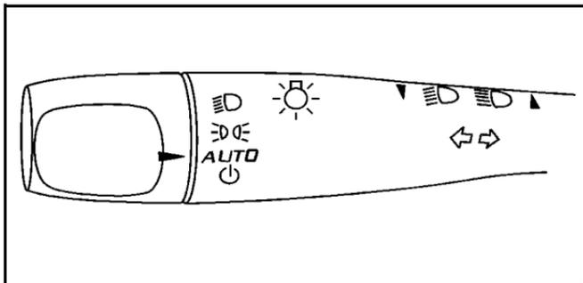
The lever on the left side of the steering column operates the following:
