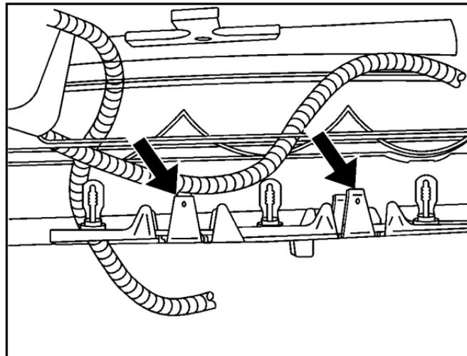
3. Pull the bulb assembly down to access the bulbs.
