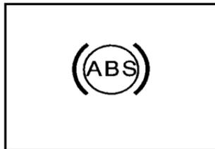
If the vehicle has ABS, this warning light on the instrument panel comes on briefly when the vehicle is started.
