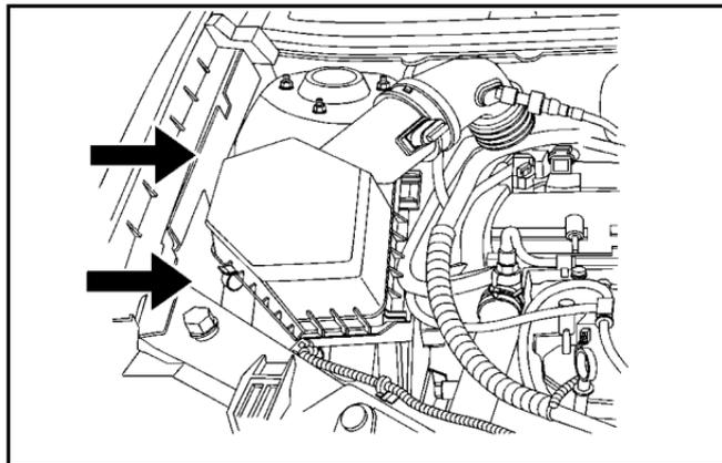
5. To remove the filter cover, unlatch the clamps, then pull up on the front and pull out.
