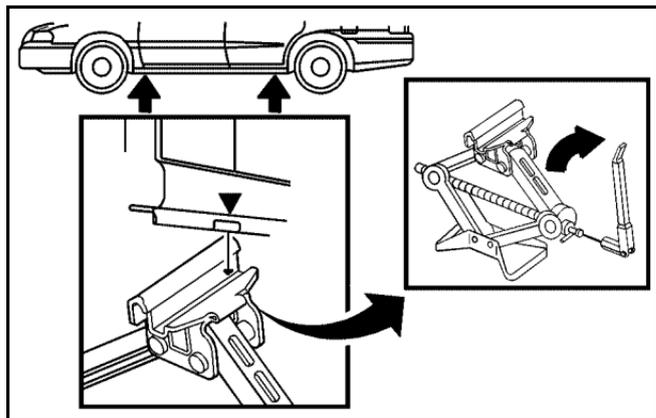
6. Position the jack lift head at the jack location nearest the flat tire. The front location is about 8 inches (20 cm) behind the front wheel opening.
