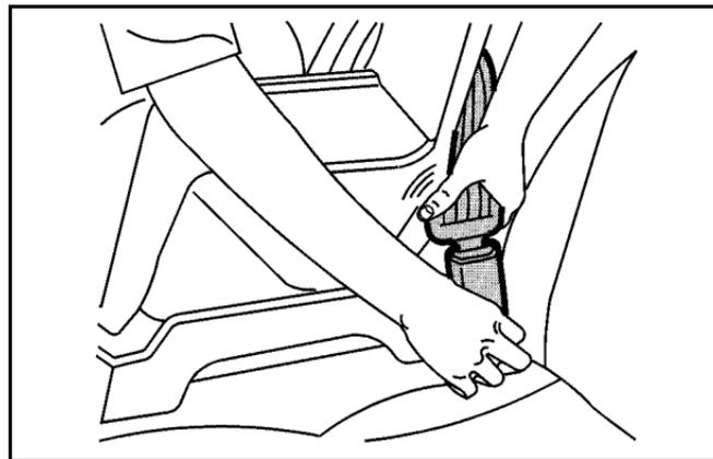
5. Push the latch plate into the buckle until it clicks. Position the release button on the buckle so that the safety belt could be quickly unbuckled if necessary.
