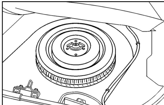
2. Lift the trunk liner to access the spare tire and tools.
