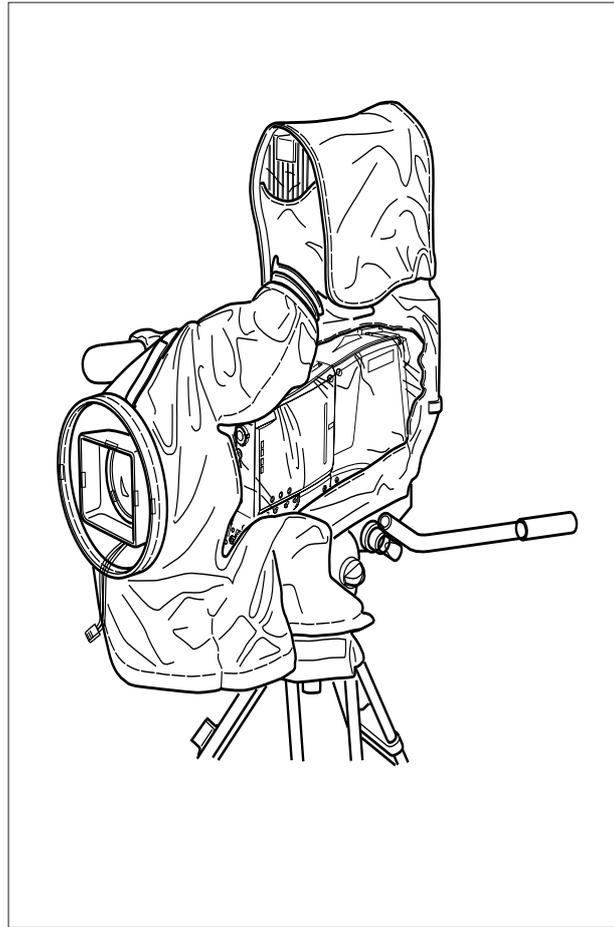
The rain and off-use cover must be used when the camera system is in a wet or damp environment. This protection is necessary for personal safety reasons. The cover can also be used indoors to protect the camera when it is used in dusty environments. It can also be useful if the camera is being put into storage. For more information on how to put on the cover refer to the User's Guide which is supplied with it.
