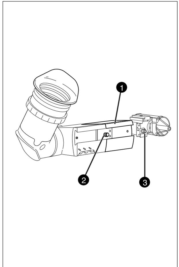
A left eye adapter is optionally available (LDK 5390/10) to allow the viewfinder to be used with the left eye.
