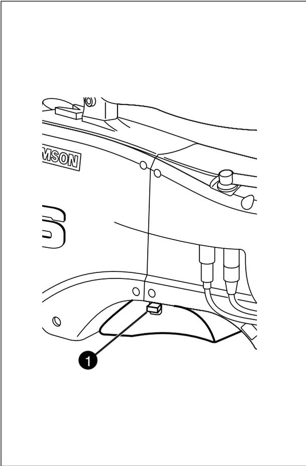
To change the position the shoulder pad press and hold lever ❶. The shoulder pad can now be moved backwards and forwards along the axis of the camera. Adjust the shoulder pad when all units have been mounted so that the best balanced position can be obtained.
