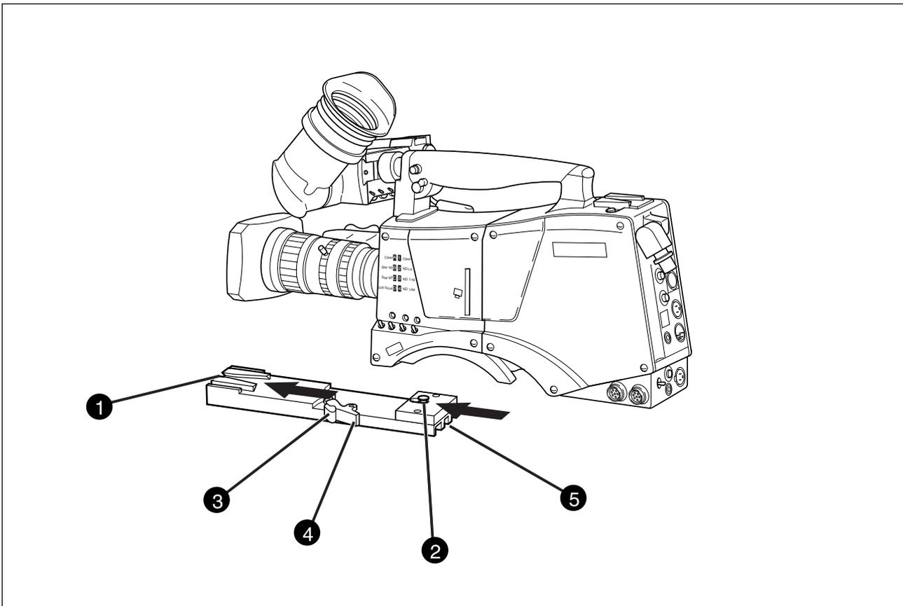
To mount the camera on a tripod, the tripod plate (LDK 530/00 is delivered as standard) must first be attached to the tripod.
