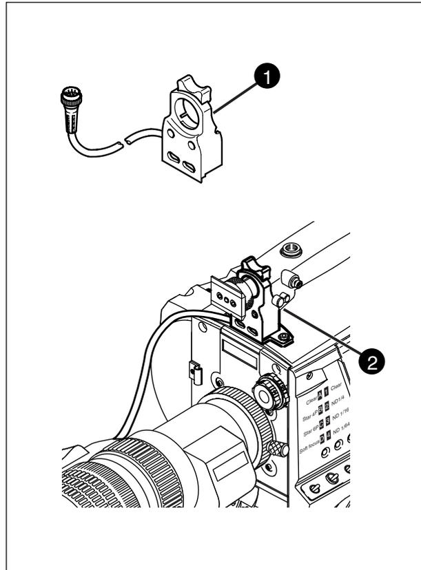
An optional zoom control unit **1** can be mounted on the carrying handle. The three available versions for different types of lens are:
