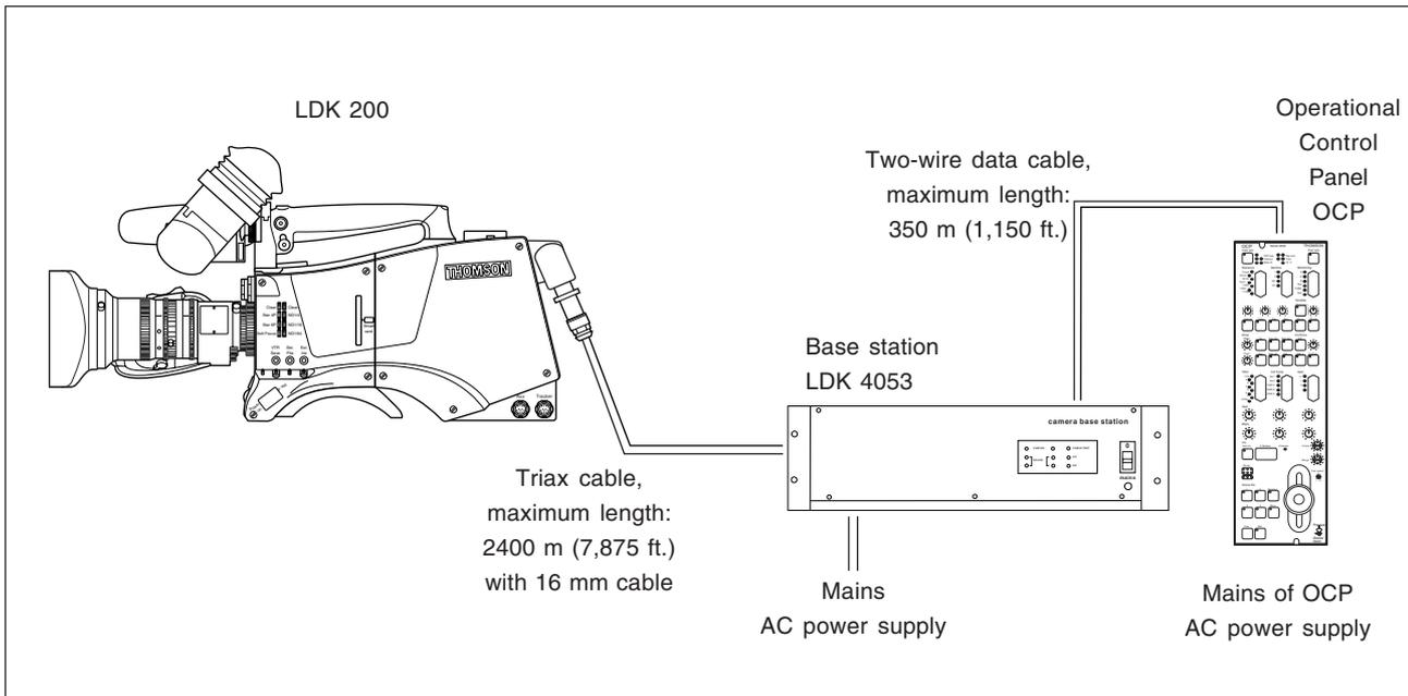
In this mode the camera is connected to a base station via a Triax adapter and cable. Remote control of the camera is achieved by a remote control panel of the Series 9000 Control System. This can be an
