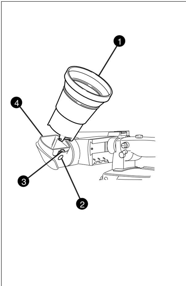
If you regularly use the viewfinder at a distance, for example, when you use the camera in the hand-held position, it is recommended that you fit the optionally available wide angle eyepiece (LDK 5390/00).
