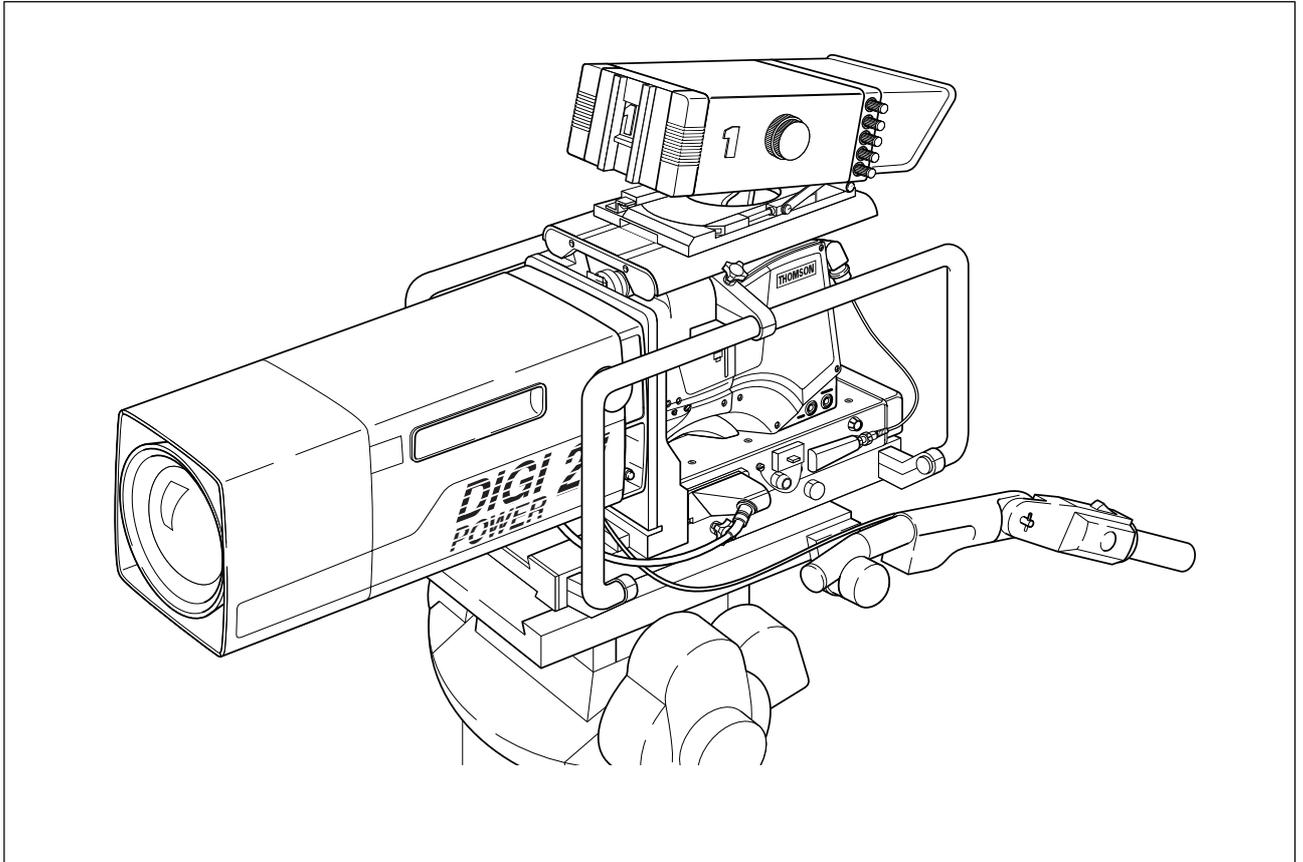
The optional SuperXPander (LDK 4482) for the LDK 100 extends the camera's use in studio and EFP situations. This adapter allows larger studio lenses and a 7-inch viewfinder to be used with the camera. Additional facilities provided include a utility power outlet and a rear control panel.
