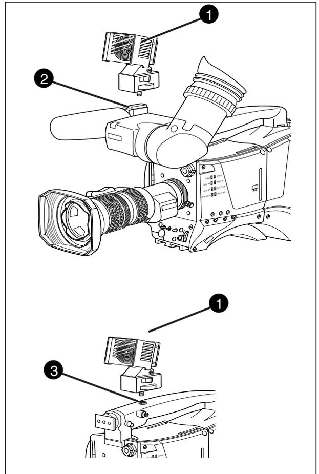
To mount a top light ① onto the camera, proceed as follows:
