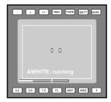
e. When the process is completed (within a few seconds) the OK message and the measured temperature appear in the viewfinder.
