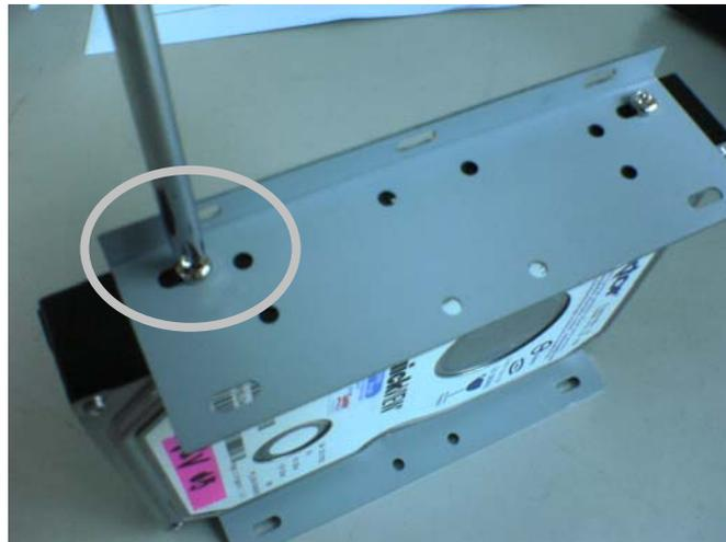
**Figure 5: Attach the HDD to the bracket**
