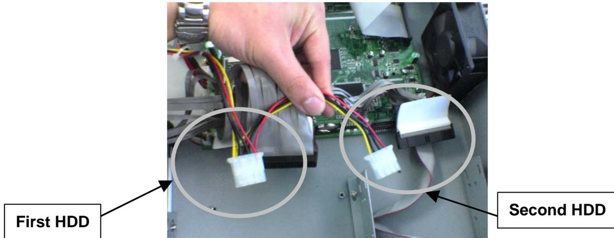
**Figure 7: Wiring the two sets of HDD's**
