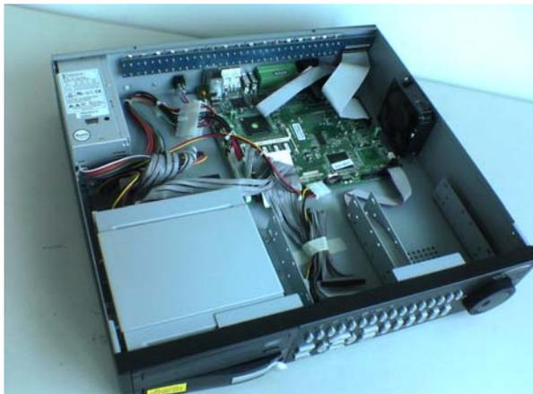
**Figure 2: Internal construction of DVR-4TN/8TN/16TN/16TS/16TT**
