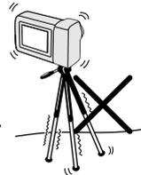
• **When using your camcorder in a cold environment, the LCD monitor screen often appears less bright immediately after the power is turned on. This is not a malfunction. To prevent the camcorder from becoming too cold, wrap it in a thick cloth (a blanket, etc.).**
