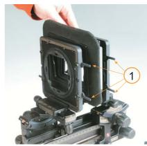
3) Mount the back plate with the standard Silvestri 4 points attachment in the back standard by using the 4 levers as explained at point 2, the plate has to be positioned with the two reference red dots one to the top and the other to the right. Sliding Back Adapters and format backs for analogue photography fit on this plate, aline the four red dots to find the position of insertion.
