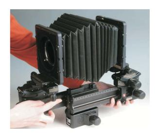
2) Now open the 4 levers (1) on the back standard and insert the bellow in its place, then close the levers until blocking the bellow; now open the 4 levers (1) on the front standard and repeat the same operation until the blocking of the bellow.
