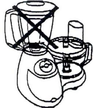
**! IMPORTANT:** Remove chopping blade protective cover before use. Chopping blade protective cover is to be used only for storage.
