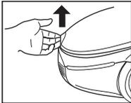
Put a finger into the cover release, and lift up to open the cover.
