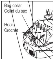
Push the bag collar in the direction of the arrows until it catches on the hooks, and then close the cover.
