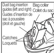
Installing a new dust bag
