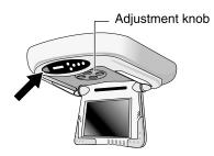
For 10.4" screens: Press the release button, as shown. The screen releases slightly and powers on automatically. Manually position it for optimal viewing.
