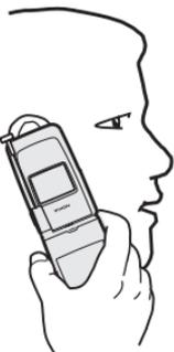
Your device has a fixed and extendable antenna located towards the top of the phone with the fold closed. Hold the phone with the antenna area pointed up and over your shoulder.
