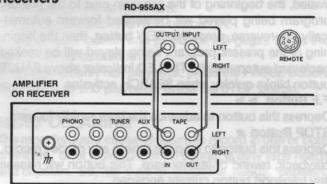
The illustration shows how the input and output terminals should be properly hooked up via the interconnect cords supplied with the unit to the Tape input and output terminals of your amplifier (integrated amplifier, preamplifier or receiver).
