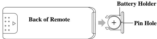
1. Turn remote over, insert a pin or straightened paper clip in the pin hole, and remove the battery holder.
