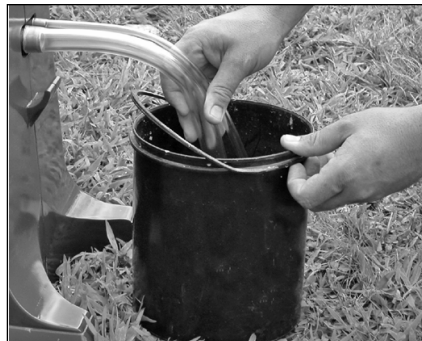
Figure 13 – Suction and bypass tubes
