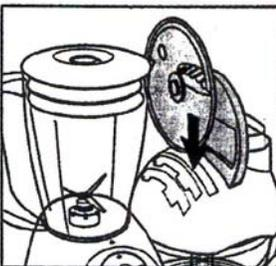
4. Place the plastic blade holder (17) & French fry blade (22) into the two longer slots.
