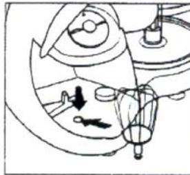
4. Push shaft of whisk beater (27) firmly into the hole.
