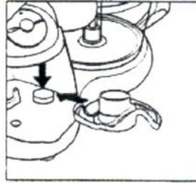
3. Place the protective cover (24) onto the chopping blade (23) and place into storage compartment. The highest part of the blade should be placed at the back of the compartment.
