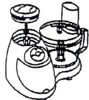
**! IMPORTANT: Remove protective chopping blade cover(s) before use. Protective blade covers to only be used for storage.**
