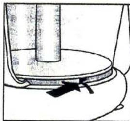
5. Fit the spindle (12) onto the motor shaft (6) and the appropriate attachments onto the spindle. Refer to the following section “Fitting & Using the Tools”.
