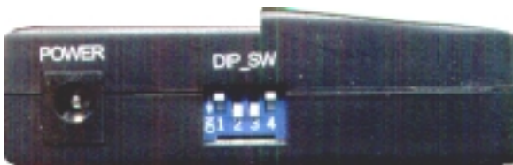
Optional Power Jack 9VDC, 500mA, Center positive DIP Switches
