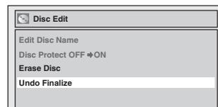
To release the finalizing for the disc, select “Undo Finalize” at step 3.
