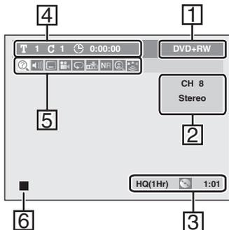
1. Indicates a disc type and a format mode. (Format mode is displayed with DVD-RW/DVD-R (Video mode) discs inserted.)
