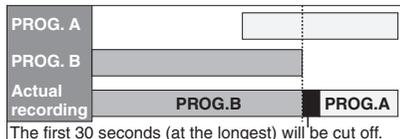
**When some programming have been made at the end time of the programming currently being recorded:**
