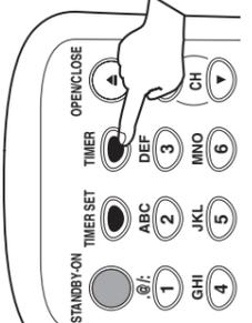
Timer Programming list appears. Select any blank line with [▲ / ▼] and press [OK].
