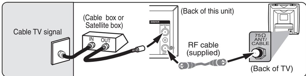
This connection allows you to view or record a scrambled channel. With this connection, channels cannot be changed on this unit. You can view or record ONLY the channels you have selected on the cable box or the satellite box.
