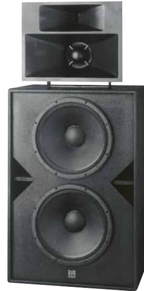
The Screen 4P is a 3-way system, with dedicated mid-range and high frequency sections. Developed by Martin Audio systems designers, this innovative solution overcomes the strenuous demands on the high frequency section of traditional 2-way cinema systems. By splitting the frequency band from 630Hz-20kHz into dedicated mid-range and high-frequency sections the Screen 4P produces superior, low distortion sound for small/medium scale cinema environments.
