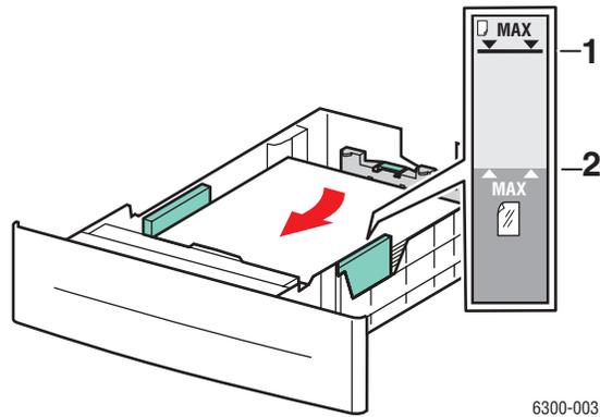
5. If necessary, press the paper guides inward to fit the paper.
