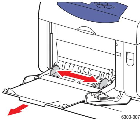
3. Insert the envelopes into Tray 1, and adjust the paper guides to fit the envelopes.
