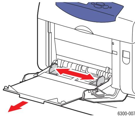
3. Insert the paper into Tray 1 (MPT), and adjust the paper guides to fit the paper.
