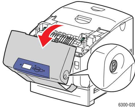
2. Pull up the two green levers at both ends of the fuser.
