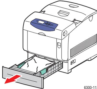
2. Remove the jammed paper from inside the printer tray slot. Confirm that all scraps of paper are removed.
