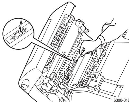
**4.** Reinstall the transfer roller.
