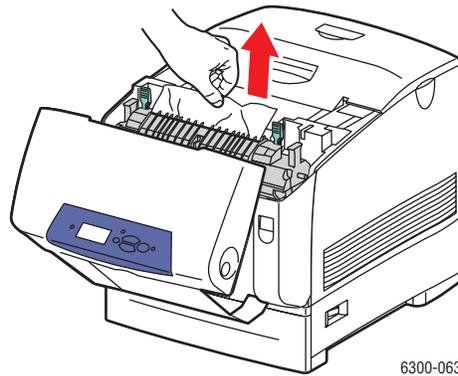
4. Completely push down the two green levers at both ends of the fuser.
