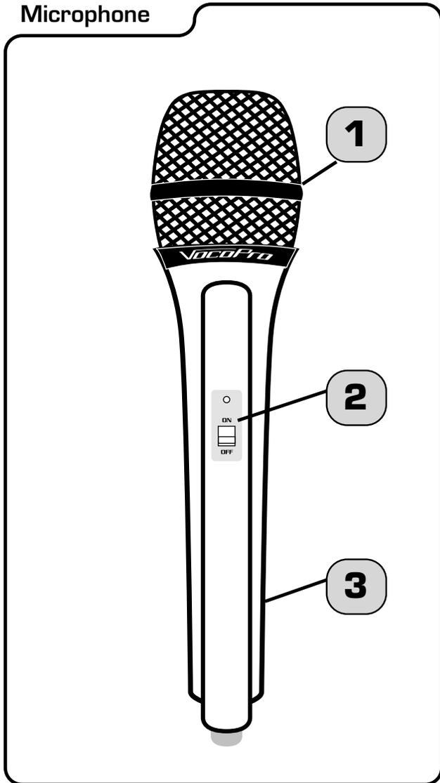
1. GRILL - Protects the microphone cartridge and helps reduce "breathy" and wind noise pick-up.
