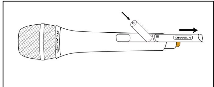
1. To remove the lid, press down on the tab and slide the lid down towards the bottom of the mic.
